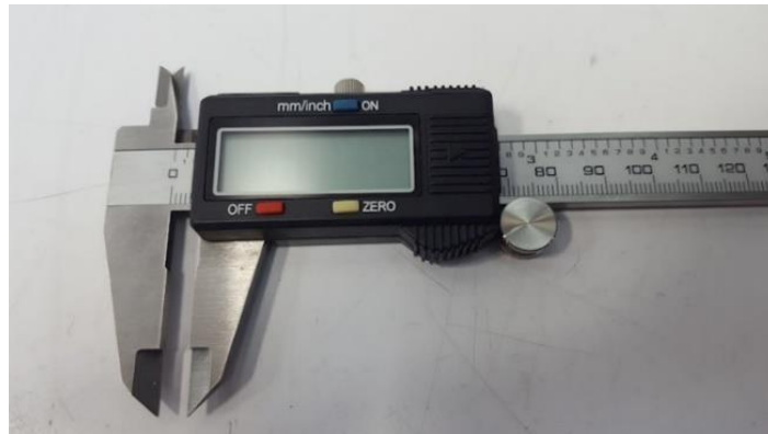
Figure 3: Digital calliper that was used to evaluate the motion of the robotic systems.
