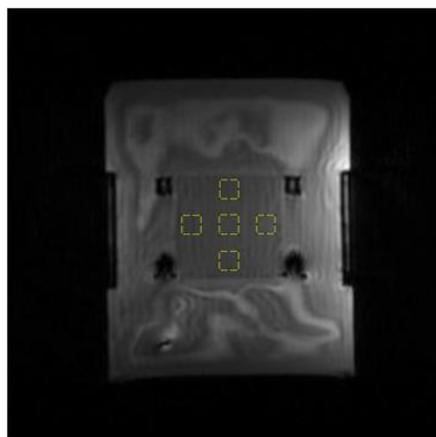
Figure 16: Standardized 5-point measurement method based on NEMA in order to calculate the NUI of the agar-based phantom for the different configurations.
