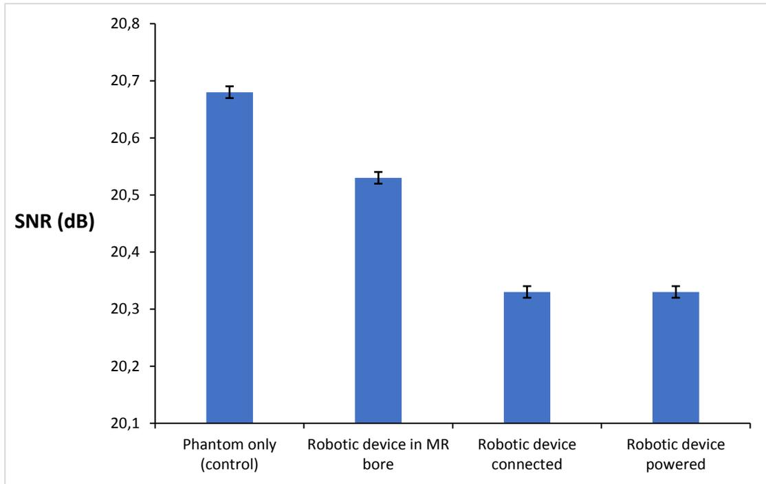
Figure 13: SNR using FSPGR sequence measured for different conditions.
