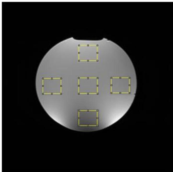
Figure 18: Standardized 5-point measurement method based on NEMA in order to calculate the NUI of the MR quality assurance phantom for the different configurations.
