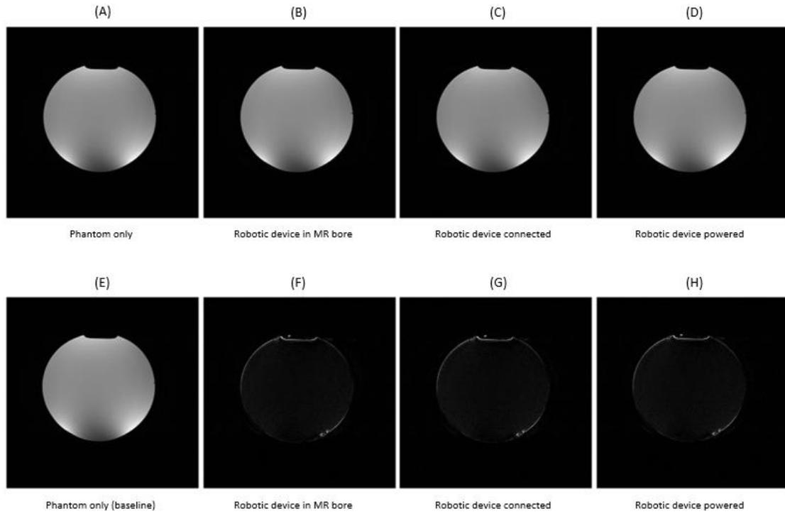
Figure 9: MR images (top) obtained using T2W-FRFSE sequence for the different conditions and the corresponding differences (bottom) between each condition and the baseline (phantom only) image.
