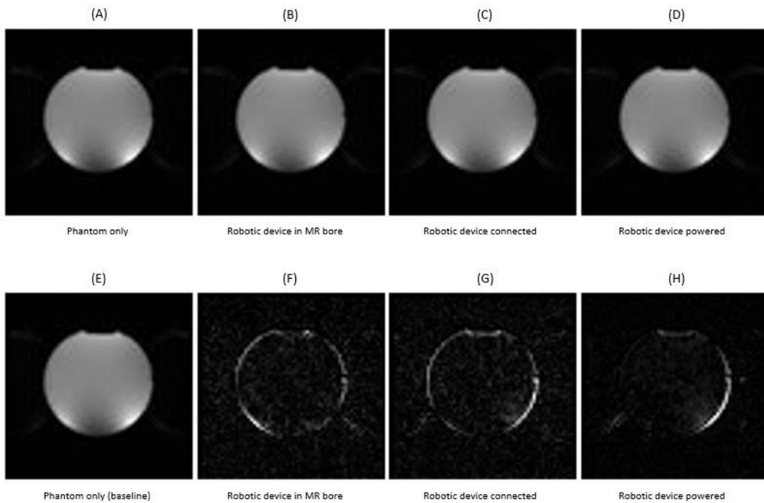
Figure 11: MR images (top) obtained using EPI sequence for the different conditions and the corresponding differences (bottom) between each condition and the baseline (phantom only) image.
