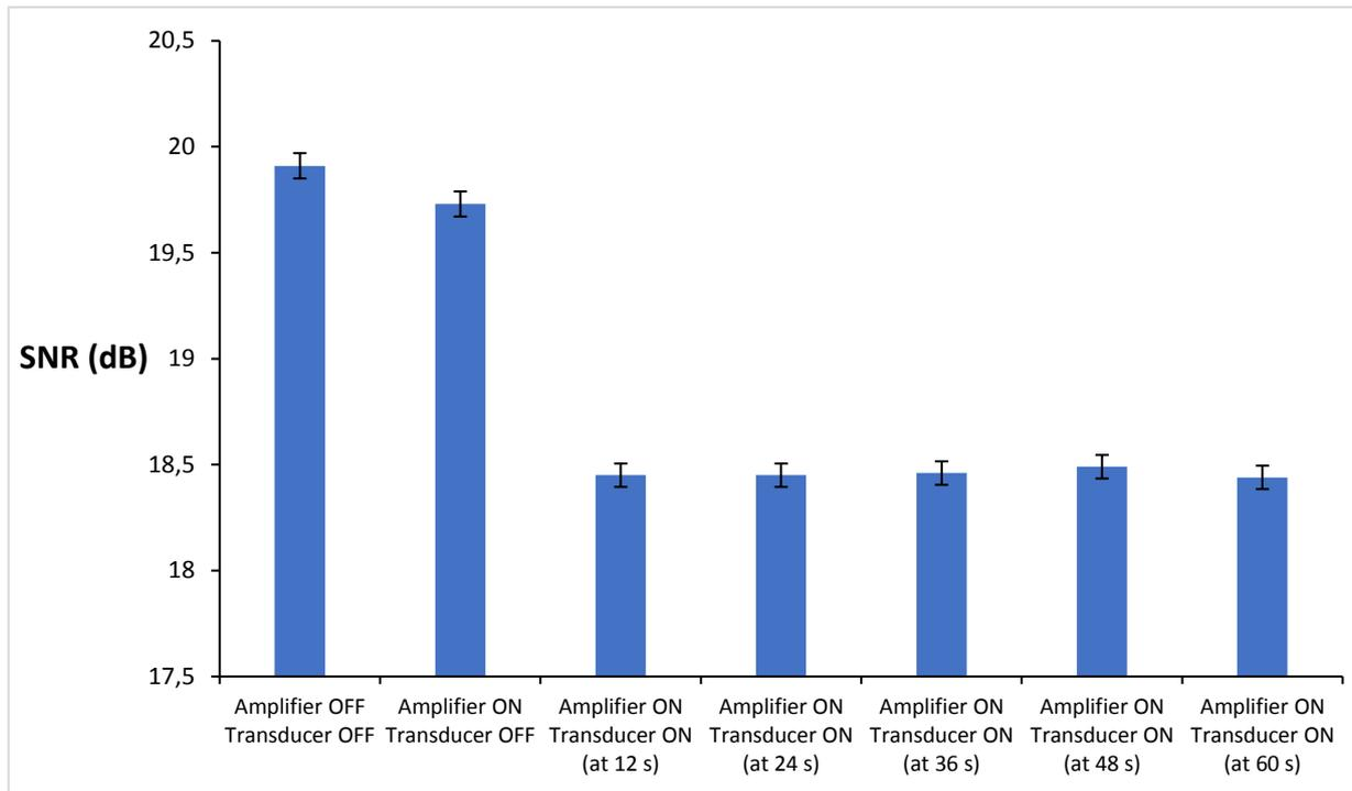
Figure 8: SNR using T1W-SPGR sequence measured for different activation conditions (RF amplifier and transducer).
