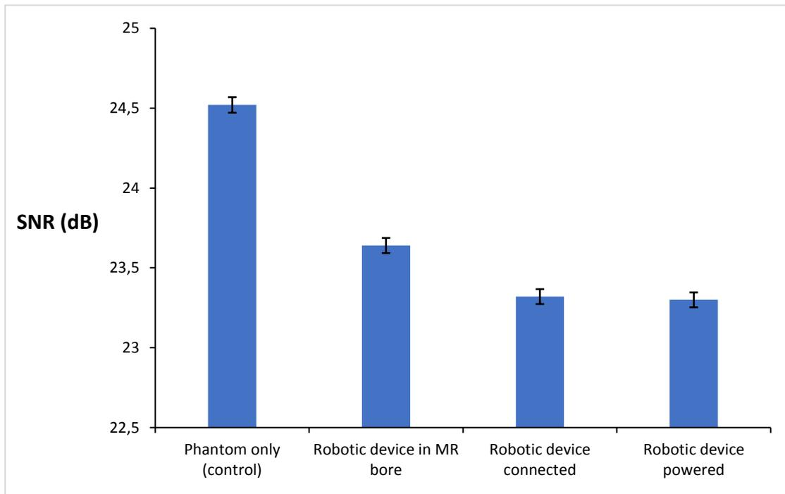
Figure 12: SNR using T2W-FRFSE sequence measured for different conditions.
