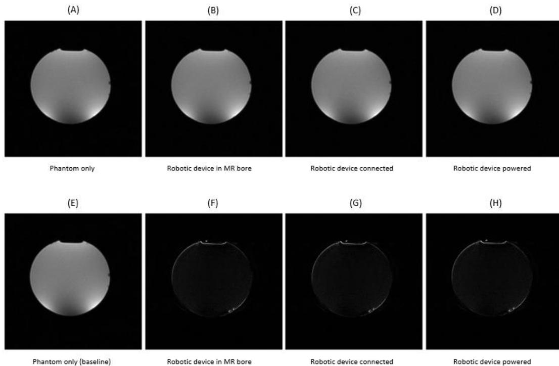
Figure 10: MR images (top) obtained using FSPGR sequence for the different conditions and the corresponding differences (bottom) between each condition and the baseline (phantom only) image.
