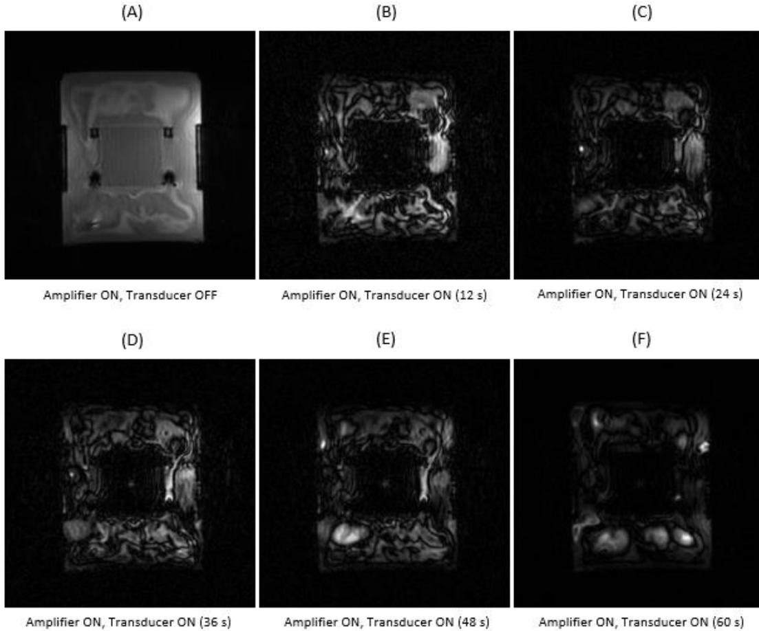
Figure 7: Difference images between the MR image obtained with the amplifier powered and transducer deactivated (A) and MR images taken with the transducer activated at 12 s, 24 s, 36 s, 48 s, and 60 s.
