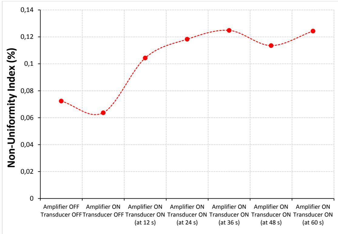
Figure 17: NUI versus different configurations using T1W-SPGR sequence for the agar-based phantom.
