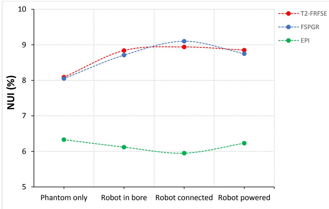
Figure 19: NUI versus condition for three MR sequences obtained in the MR quality assurance phantom.
