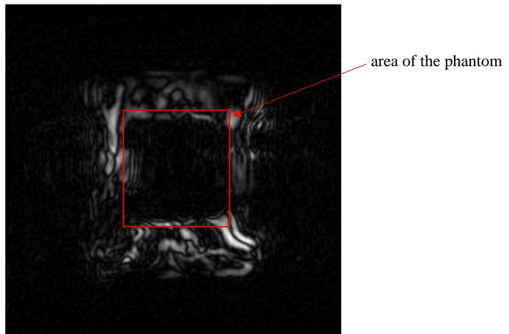
Figure 6: Difference image between the MR image obtained with the amplifier deactivated and the MR image obtained after powering on the amplifier.
