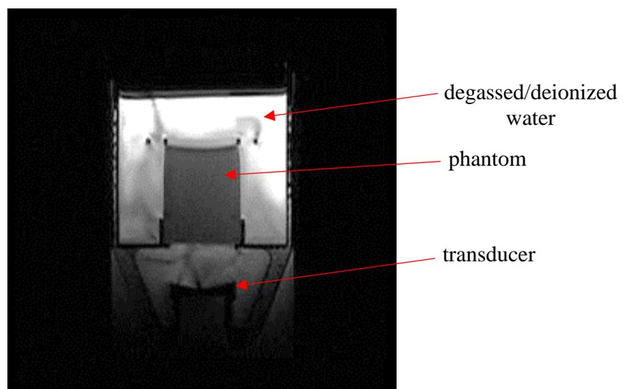
Figure 4: T2W-FSPGR coronal image of the experimental set-up that was used to investigate the MR compatibility of the transducer.
