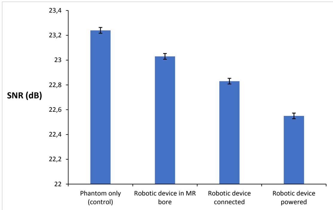
Figure 14: SNR using EPI sequence measured for different conditions.
