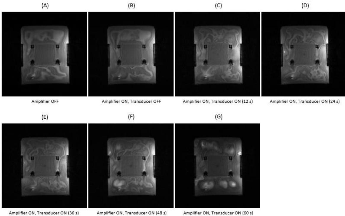
Figure 5: Coronal MR images obtained using T2W-SPGR sequence for A) amplifier without DC supply, B) amplifier with DC supply and transducer deactivated, C) amplifier with DC supply and transducer activated at 12 s, D) 24 s, E) 36 s, F) 48 s, and F) 60 s .
