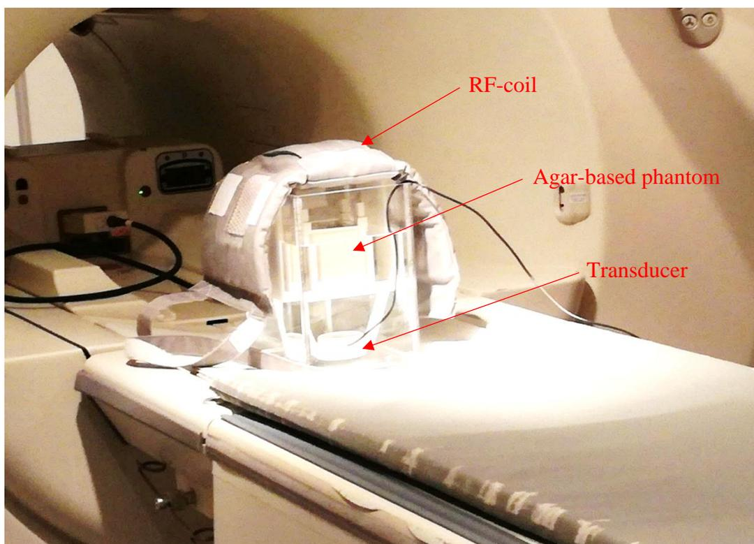
Figure 1: Experimental set-up to check the MR compatibility of the transducer and amplifier activation.
