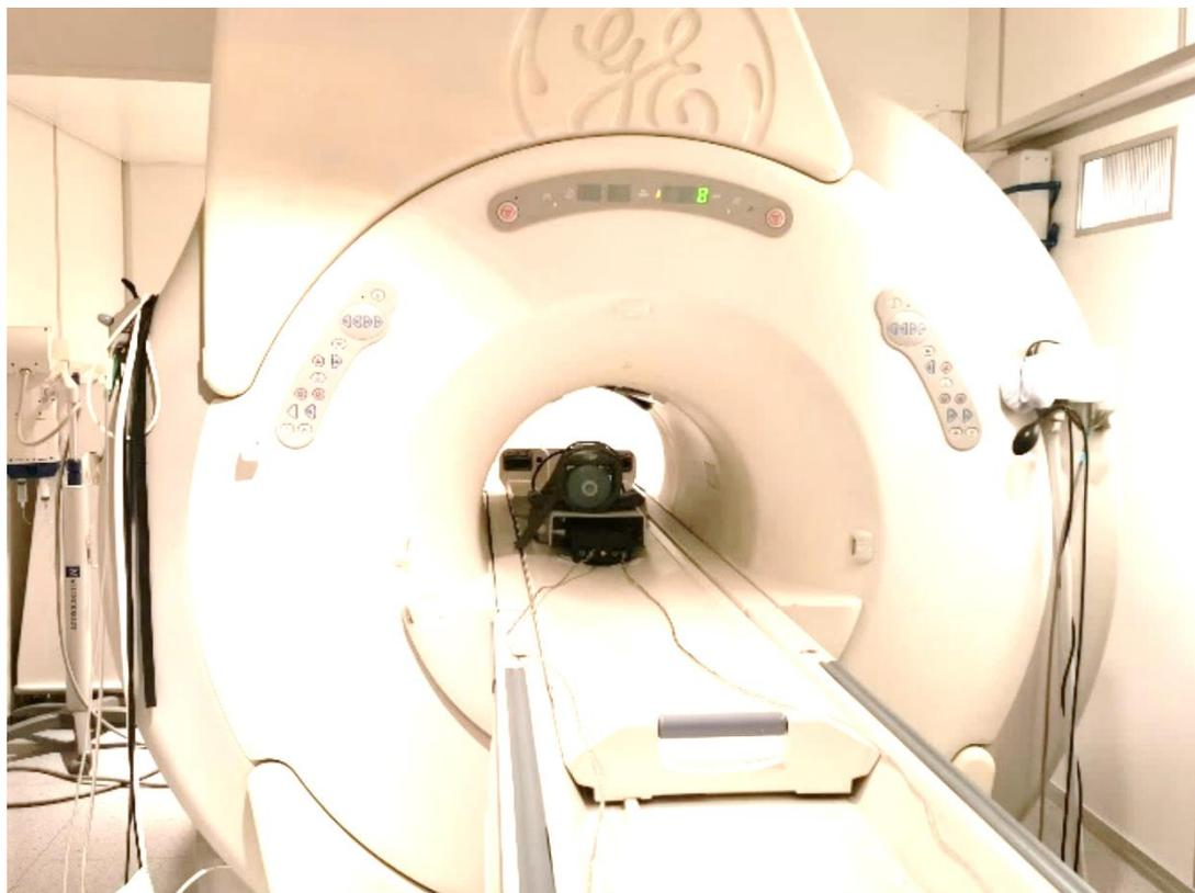
Figure 3: Experimental set-up as illustrated in the MR bore in order to check the MR compatibility of the piezoelectric motors and optical encoders. The 2 DOF robotic system was used.
