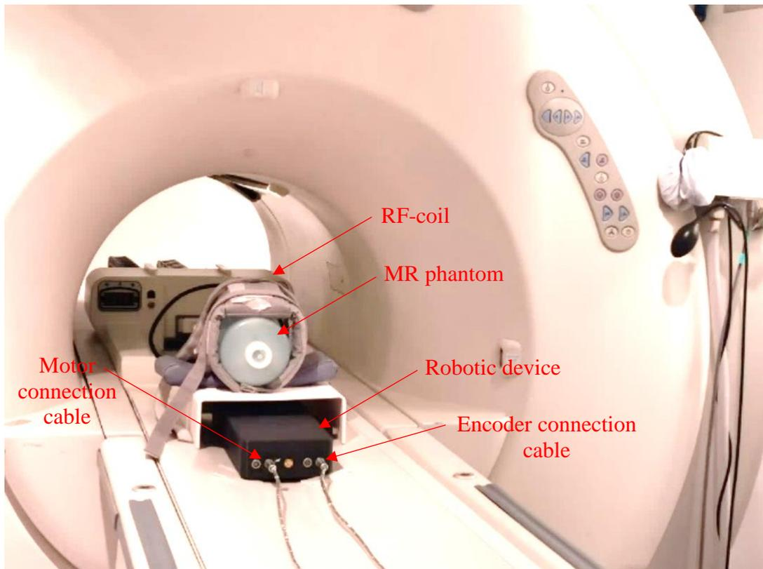
Figure 2: Experimental set-up as illustrated in the MRI room but outside the MR bore in order to check the MR compatibility of the piezoelectric motors and optical encoders. The 2 DOF robotic system was used.
