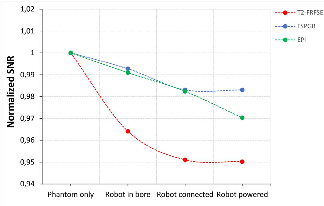
Figure 15: SNR for three MR imaging protocols with the system in different configurations. Lines represent mean SNR.
