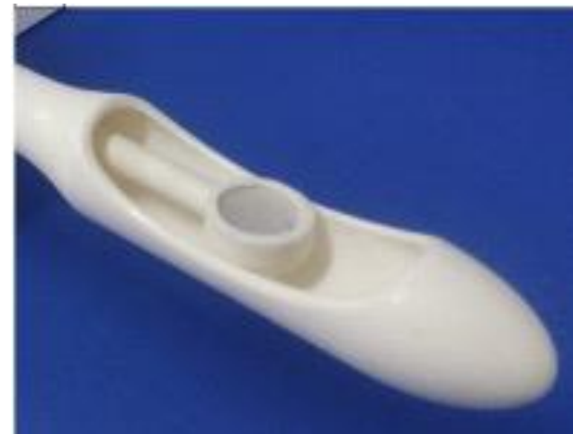
Figure 4: Photo of the manufactured transducer inside the probe.
