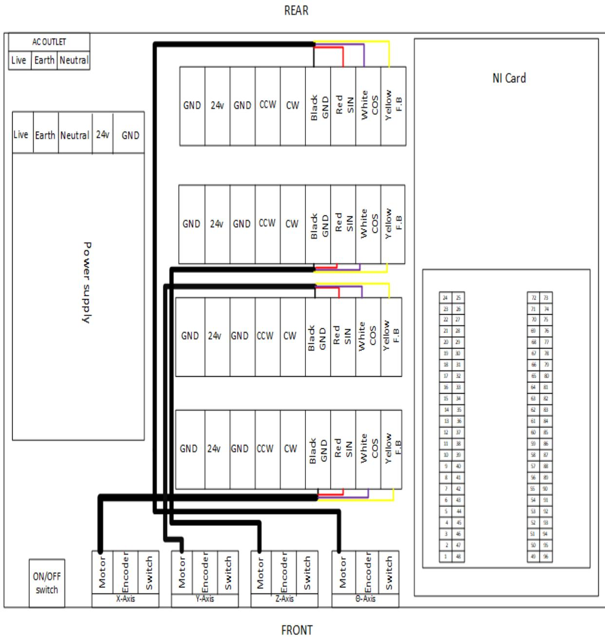
Figure 5: Connection between the motor driver and the motor.
