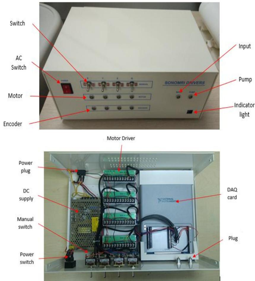
Figure 3: A) Photo of the electronic system. B) The electronic components installed in the system.
