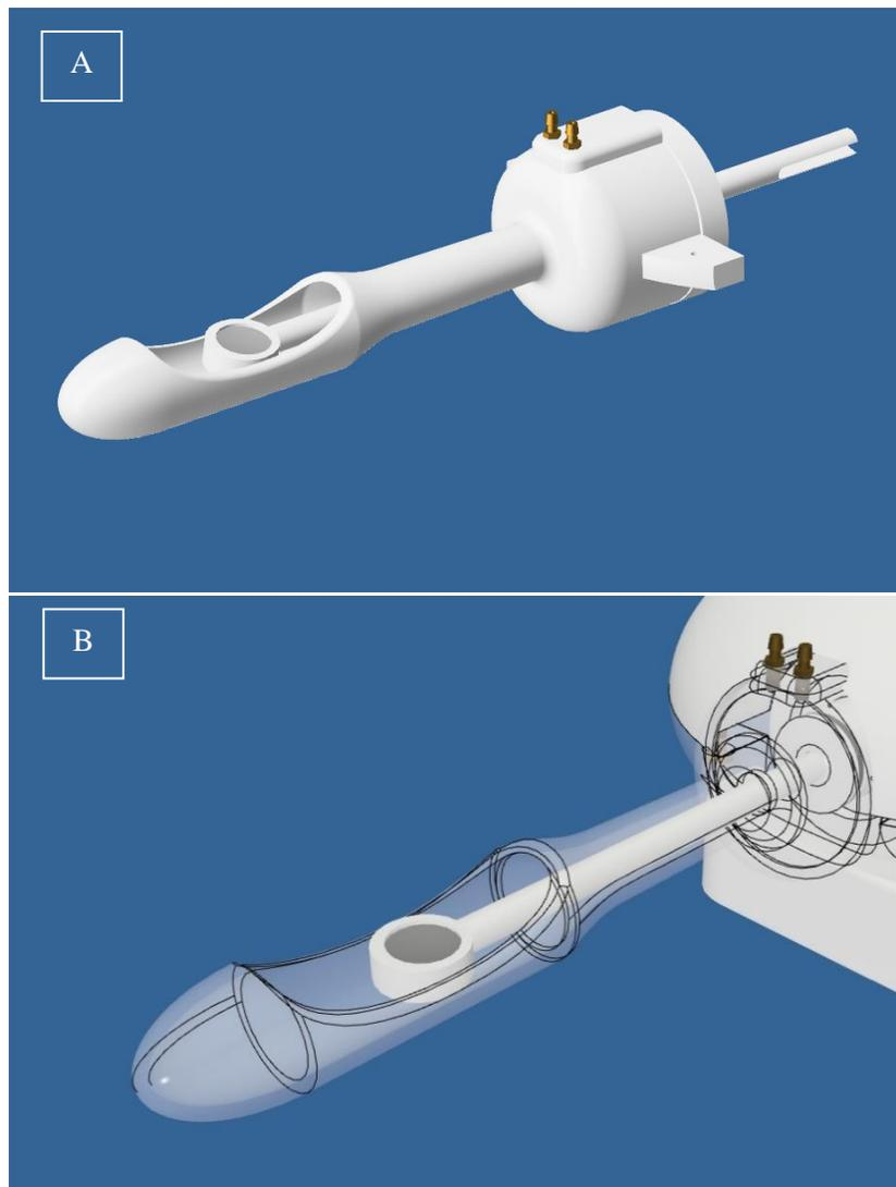
Figure 2: A) CAD drawing of the transducer probe assembly. B) Transparent view of the probe demonstrates the mechanism.
