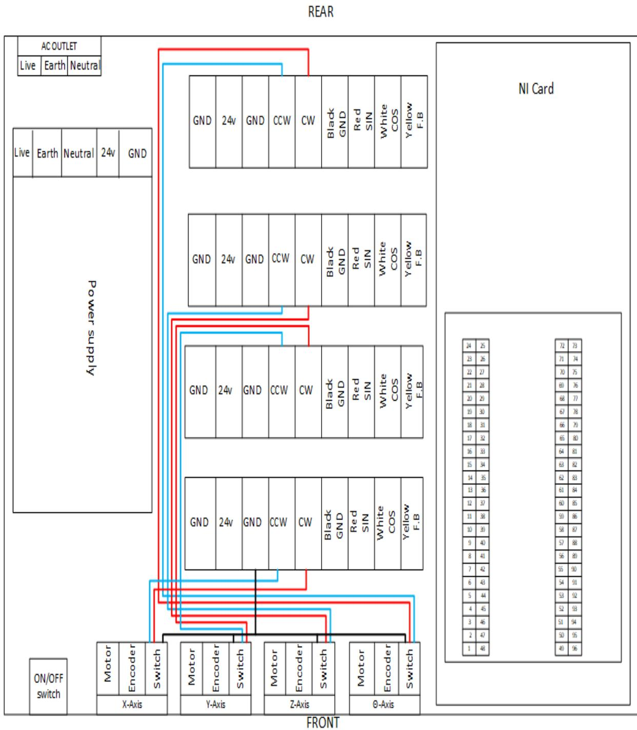
Figure 6: Connection between the manual switch and the motor driver.
