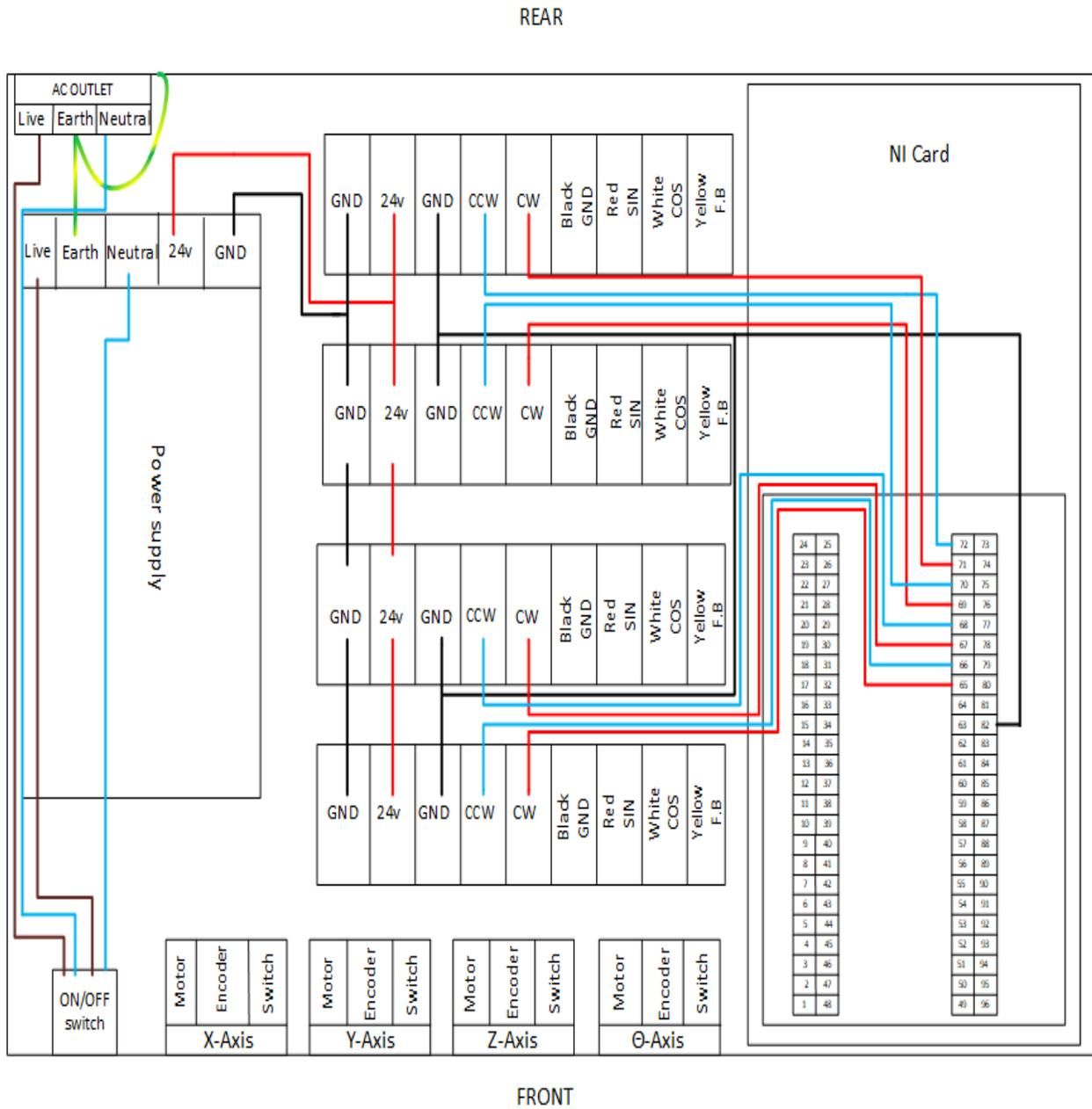
Figure 4: Connection between the motor driver and the data acquisition card.
